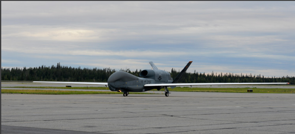
The RQ-4 Global Hawk is a high-altitude, long-endurance, unmanned aircraft system with sensors that provide intelligence, surveillance, and reconnaissance capability.
