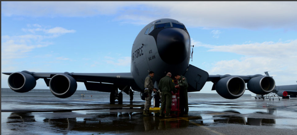
The KC-135 Stratotanker is an aerial refueling and airlift aircraft. KC-135s provide aerial refueling support to Air Force, Navy, Marine Corps, and allied nation aircraft and transport litter and ambulatory patients during aeromedical evacuations.
