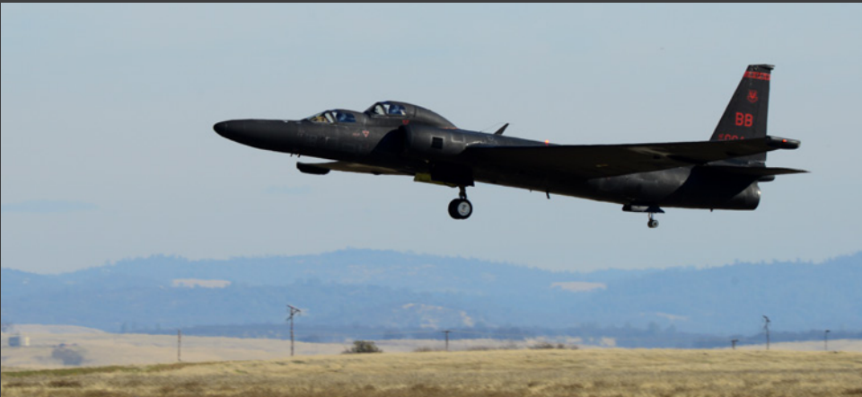
The U-2S Dragon Lady is a single-seat, single-engine, high-altitude reconnaissance and surveillance aircraft that provides signals, imagery, and electronic intelligence. Long and narrow wings give the U-2 glider-like characteristics and allow it to quickly lift heavy sensor payloads to altitudes over 70,000 feet, keeping them there for extended periods of time. Shown here is the two-seat TU-2S variant used to train pilots.
