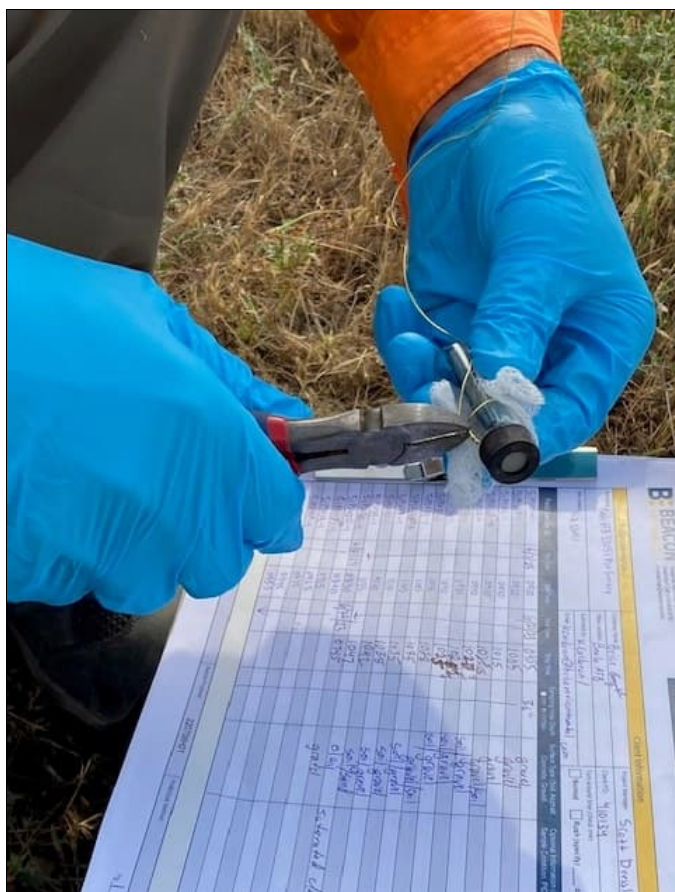
Snipping off the suspension wire after retrieving the passive soil gas sample.
