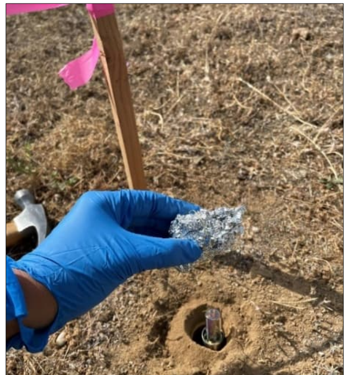
Installing a passive sampler with aluminum seal for the passive soil gas survey.
