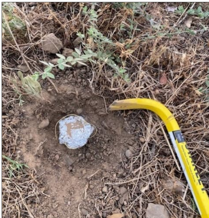
Removing a passive sampler after being left in the ground for 14 days.
