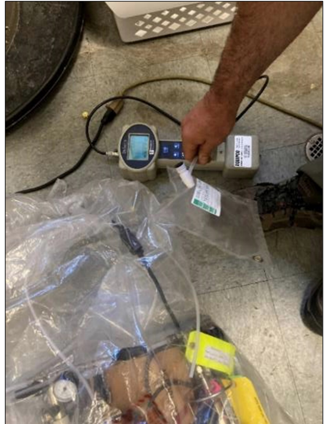
Sub-Slab Vapor Sampling
