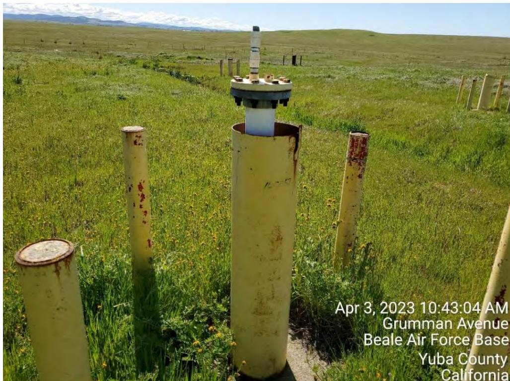
Photo C-2. CG041-010 (SD010) – ERD (EVO injections) for wells exhibiting rebound
