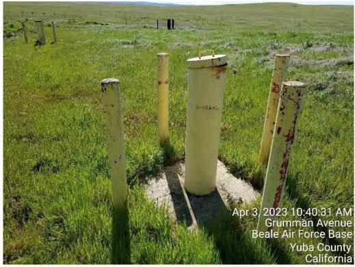
Photo C-1. CG041-010 (SD010) –Monitoring wells in the foreground and background (EA monitoring)
