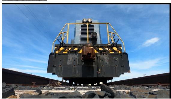
U.S. Air Force locomotive 1668 travels on the railroad tracks at Beale Air Force Base, California, to pick up a fuel shipment on March 5, 2025. By continuing to operate this General Electric 80-ton switcher, Beale saves time and resources by transporting approximately 4 fuel trucks worth of jet fuel onto base at once. (U.S. Air Force photo by Charles Borsos)
